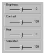
Dragging a slider to the left decreases the level and to the right increases it. The number at the right of each slider displays the brightness (value range: -100 to 100, default: 0), contrast (0 to 200, default: 100), hue (-180 to 180, default: 0), or saturation value (0 to 200, default: 100).
